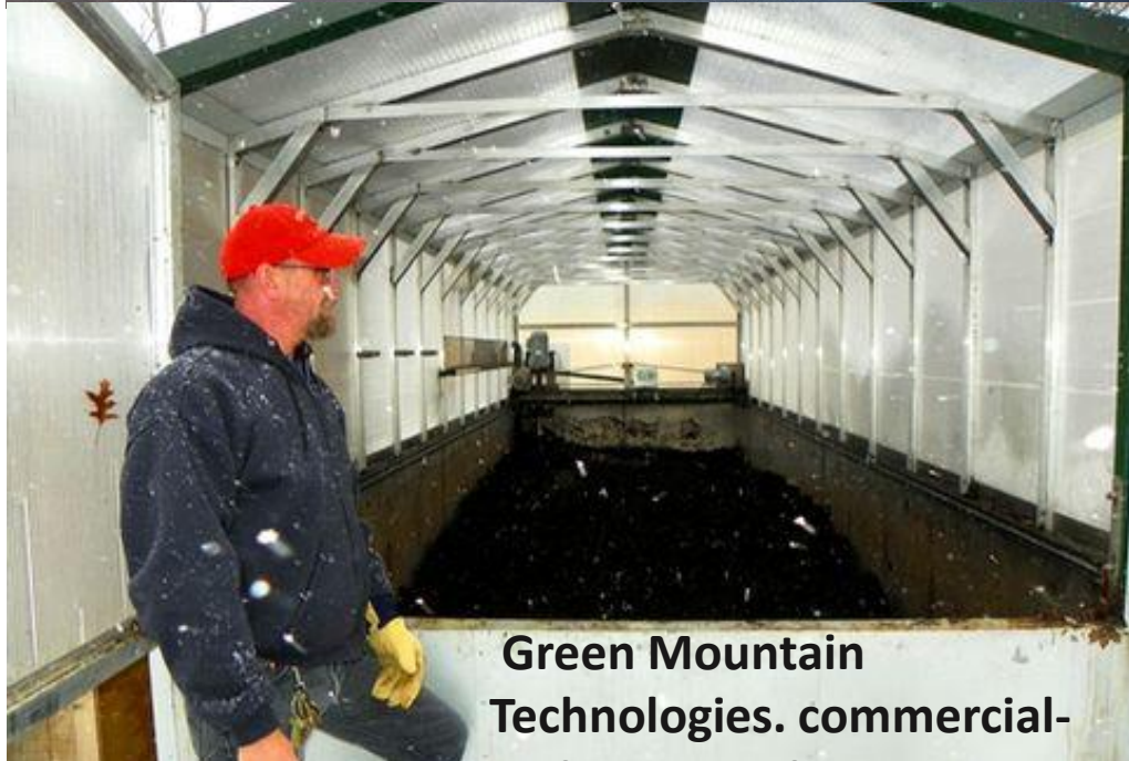
Biofiltration of air to scrub odors
