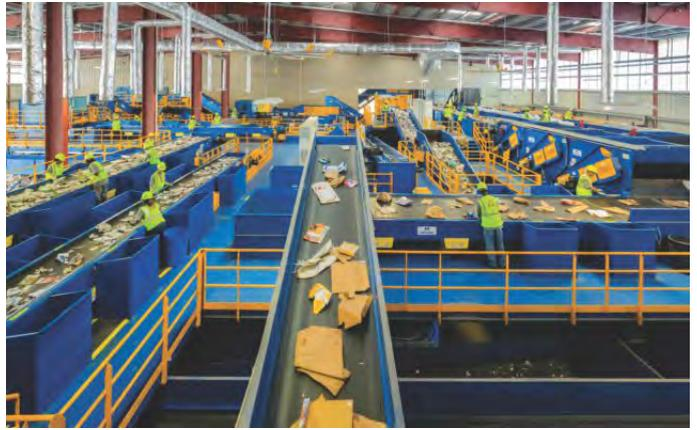
Improved MRF uses several mechanized processes; minimizing hand sorting, while maximizing diversion.
