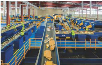
Improved MRF uses several mechanized processes; minimizing hand sorting, while maximizing diversion.
