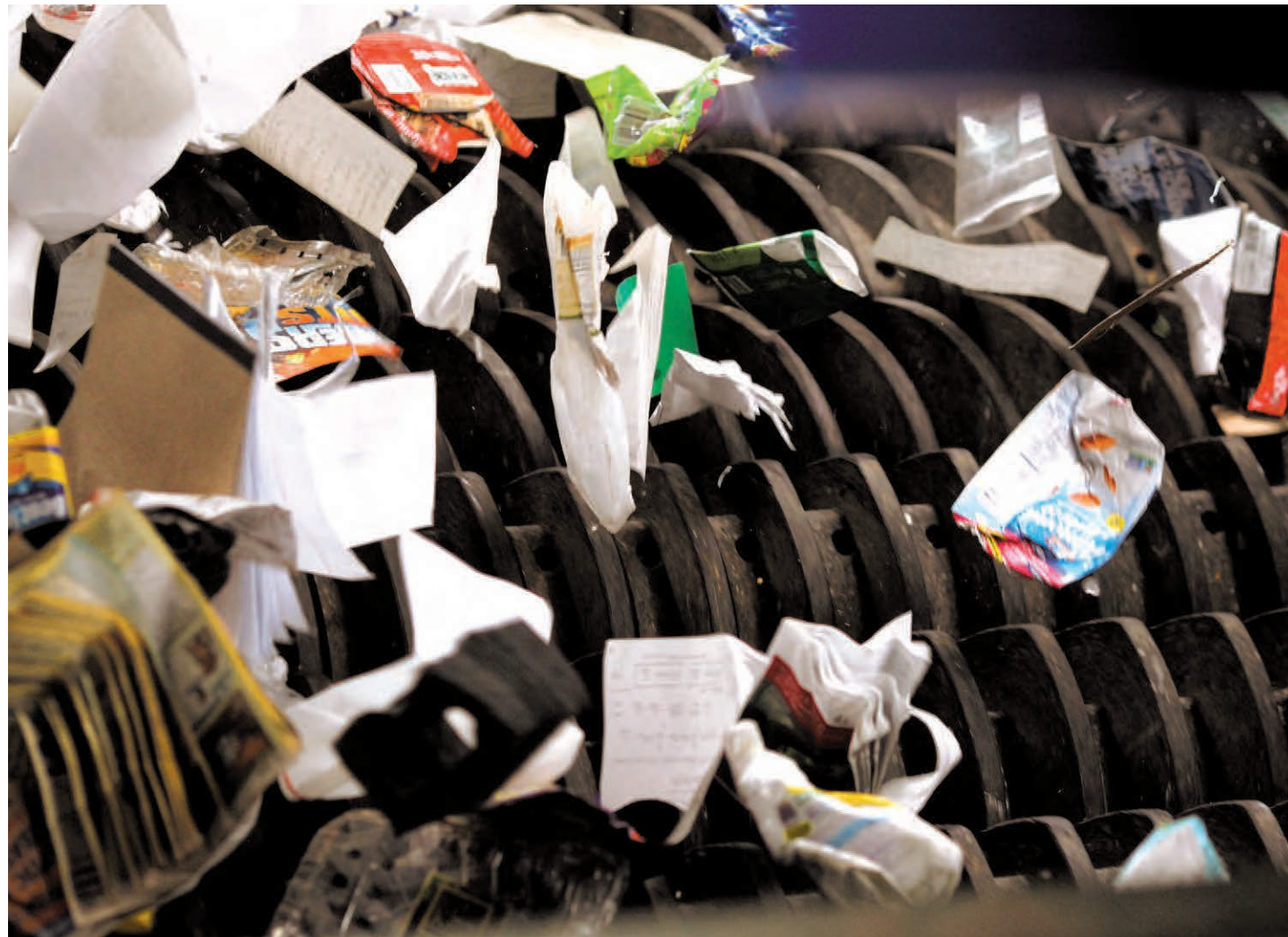
Rotating gears at MRF 2.0 move paper up a ladder, separating it from three-dimensional objects—i.e., anything other than paper.
